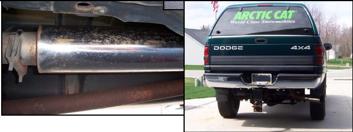
This is a 409 stainless steel system with a T304 tip - 11 months old. Truck resides in Michigan.
